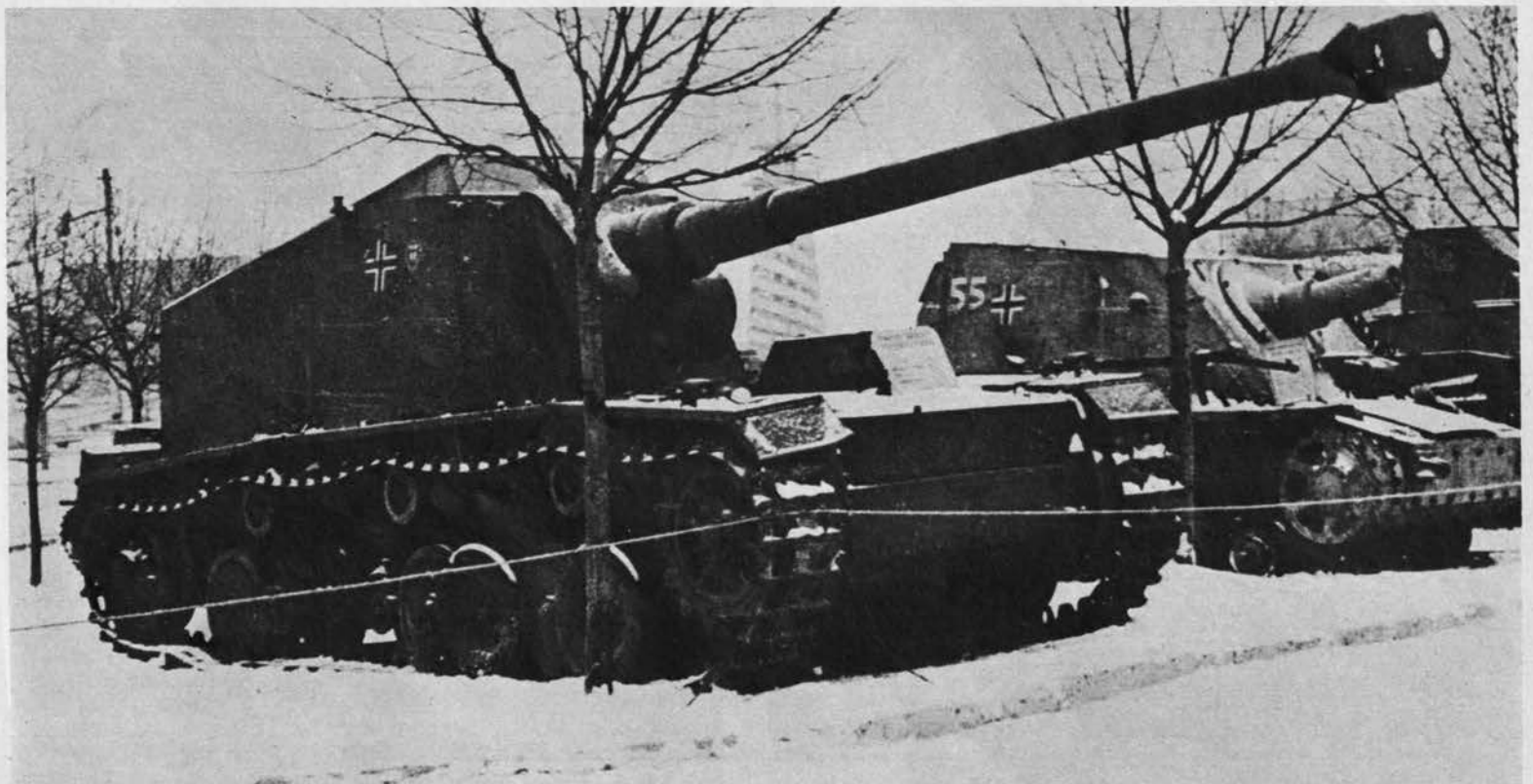
Huge 128-mm. gun displayed here is mounted on a modified PzKw VI chassis which has the usual overlapping bogie wheels and three re-
